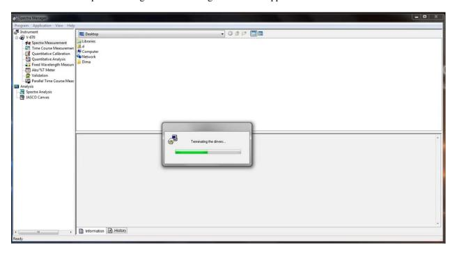
d. Only after the drivers have been terminated switch off the instrument.
